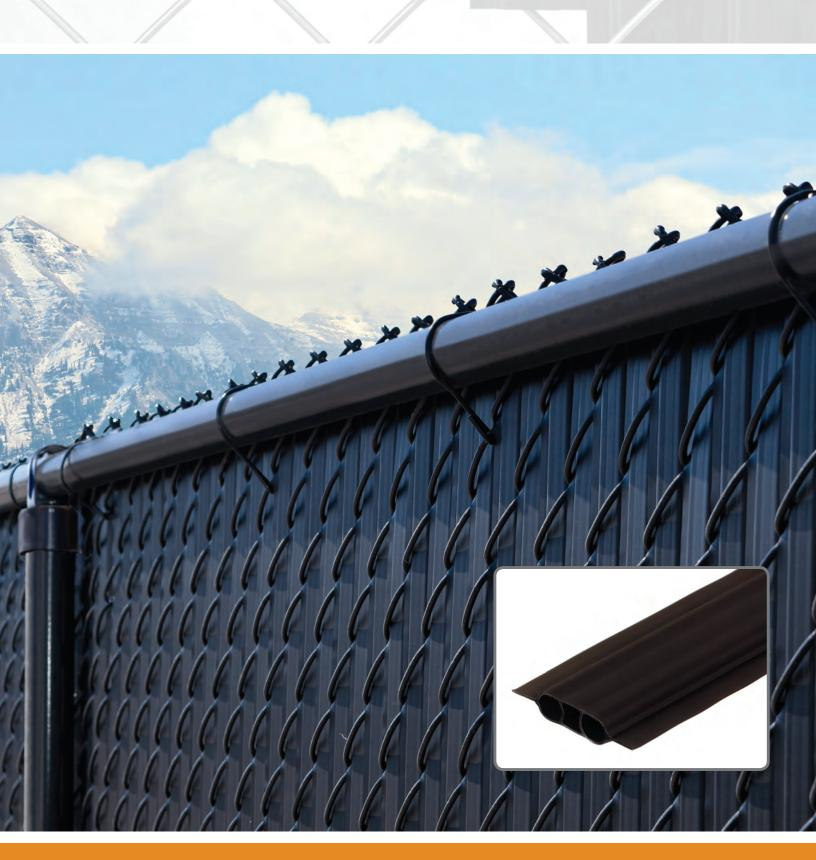
The SoliTube™ Slat product, exclusively from Slat Warehouse, is designed to provide maximum privacy in 2" chain link mesh. The body of the SoliTube™ Slat is a double-wall, flat tubular extrusion formulated in High Density Polyethylene (HDPE), with properties and additives to ensure color and functionality for many years. The privacy fins on each side, are formulated with a durable, yet flexible, Thermal Plastic Elastomer (TPE) which gently molds around the knuckles formed in the chain
